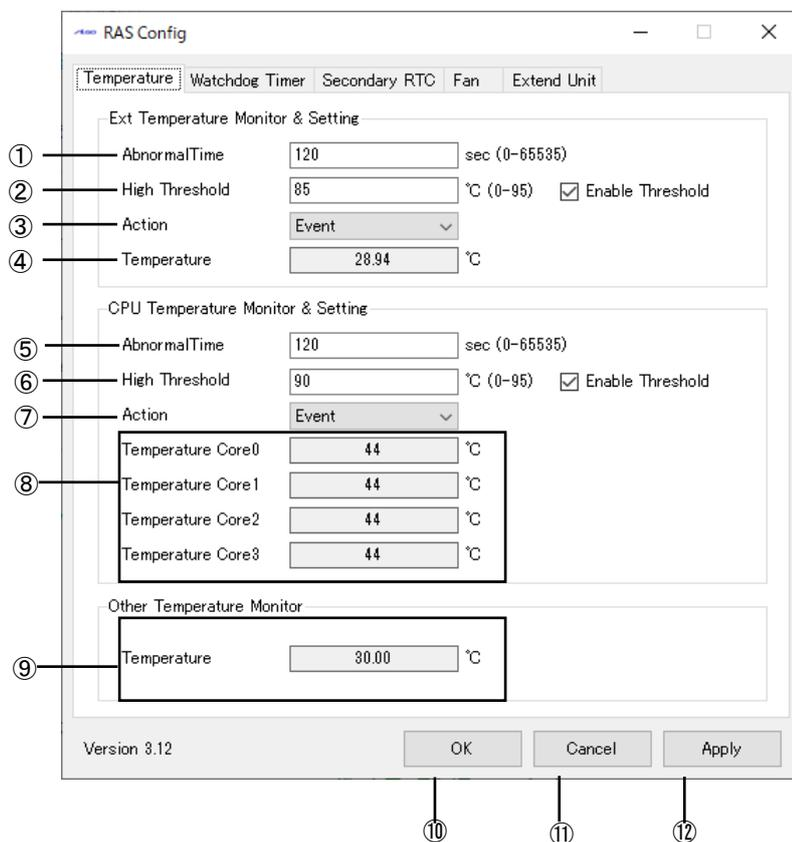
図 2-11-3-1. Temperature Configuration
