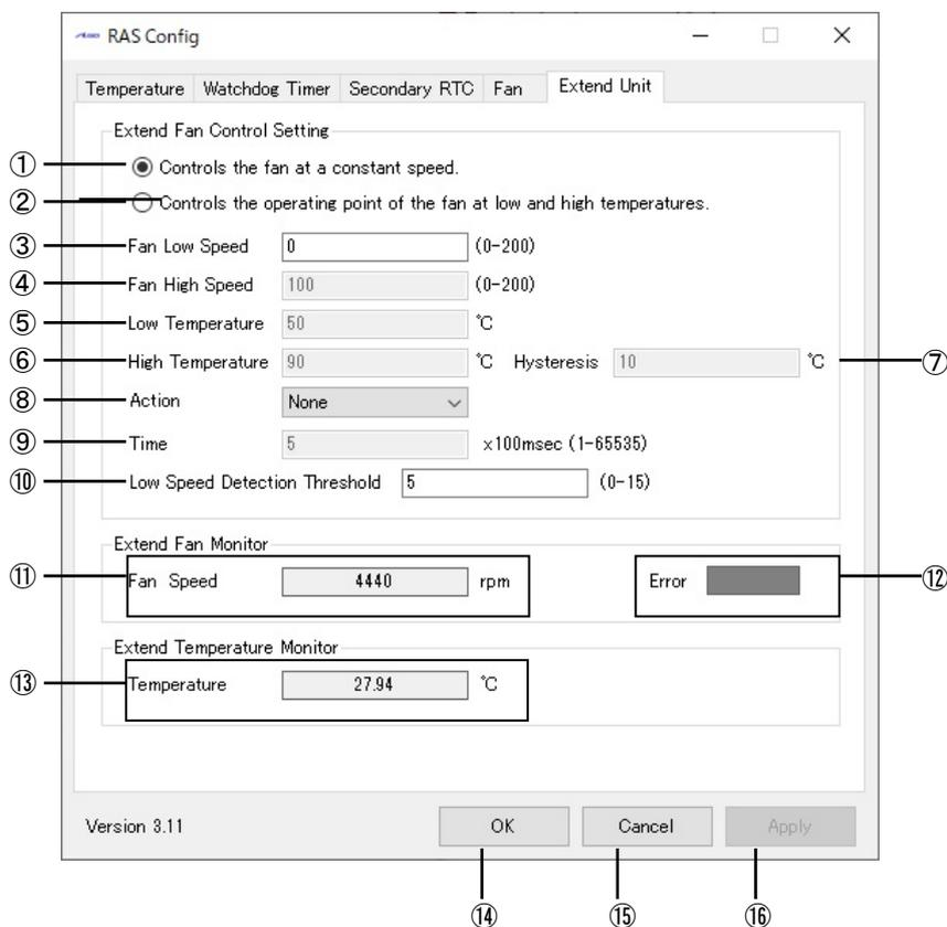
図 2-11-11-1. Extend Unit Configuration
